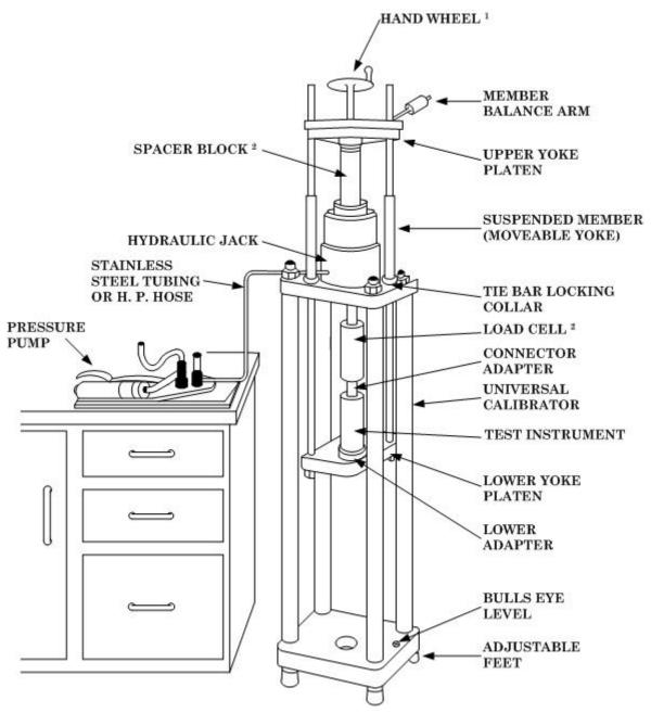
$<sup>^{\</sup>rm l}\,\mbox{On some models}$  of CALIBRATOR, the handwheel is replaced by an electric motor
